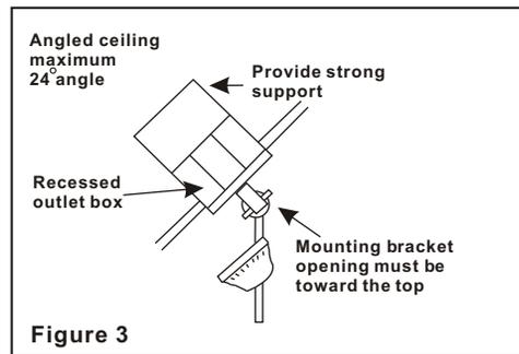
**Note:** You may need a longer downrod to maintain proper blade clearance when installing on a steep, sloped ceiling.
