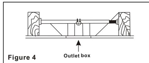
To hang your fan where there is an existing fixture but no ceiling joist, you may need an installation hanger bar as shown in Figure 4 (available at your Hampton Bay Retailer).
